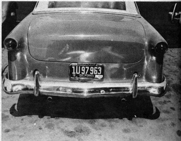
(Above) View of Ford after shaving deck and revamping tail lights.
