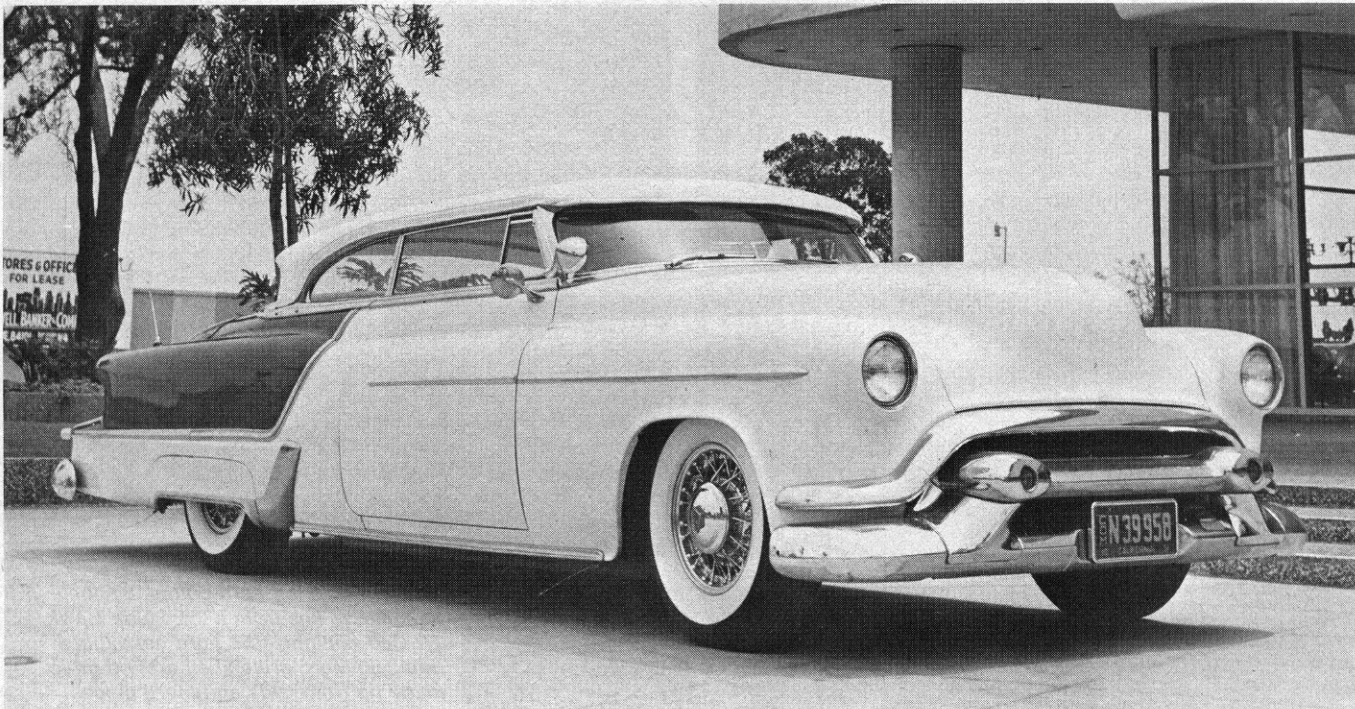
Jerry Brownstein's '53 Olds 98 by Gaylord was lowered three inches in front by cutting the coil springs, and four inches in back by X-ing the frame. The soft top is removable. The rear body has been extended 14 inches to go behind the continental kit.
