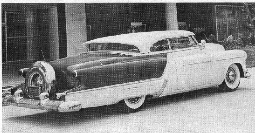
Dana Boller's '49 Ford 2-door is example of thoughtful customizing. It was sectioned, hood and deck were de-chromed, headlights Frenched, parking and taillights set into bumper guards, door handles removed and a simple straight-bar grille added.
