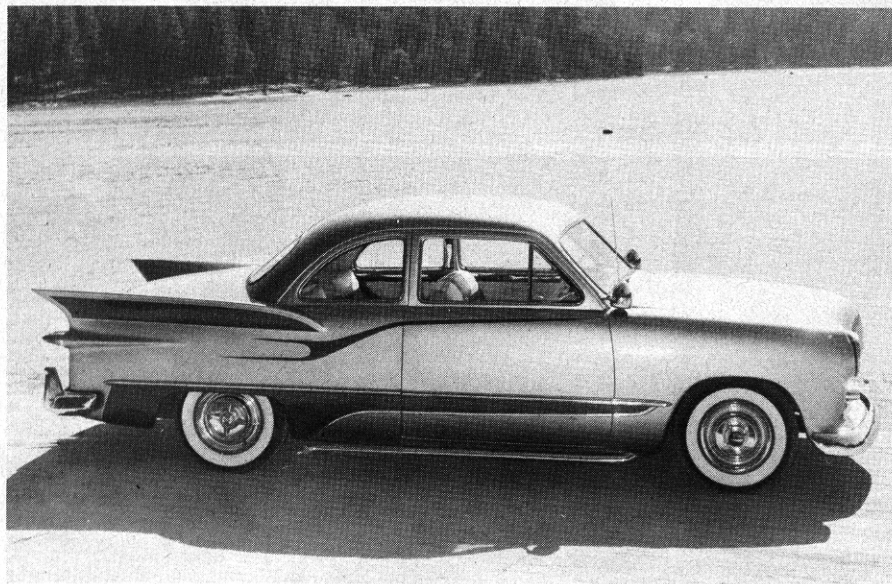
Jere Ehrich's '50 Ford coupe, by Joe Bailon, has fins from a '57 Stude Hawk, '59 Cad taillights, '54 Ford headlight rims, '50 Merc grille shell around grille made up from Olds and Merc pieces, and DeSoto side trim. Car is lowered four inches and painted Pagan Gold with candy apple trim.
