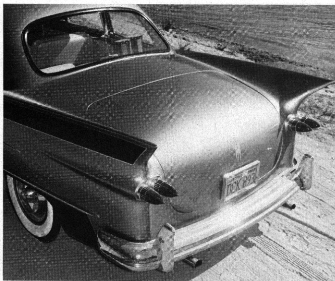
Jere Ehrich's '50 Ford coupe, by Joe Bailon, has fins from a '57 Stude Hawk, '59 Cad taillights, '54 Ford headlight rims, '50 Merc grille shell around grille made up from Olds and Merc pieces, and DeSoto side trim. Car is lowered four inches and painted Pagan Gold with candy apple trim.
