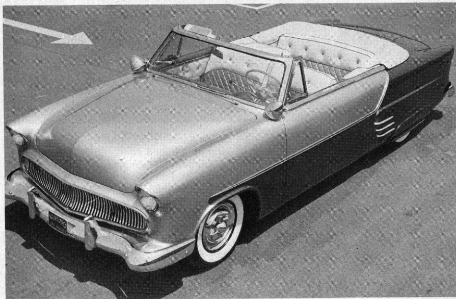
Merc convertible (1940) was lowered, de-chromed, and the taillights faired into the fenders, which had Buick skirts installed. Crowning glory was a removable hard top which faired nicely into back of body. See page 40.
