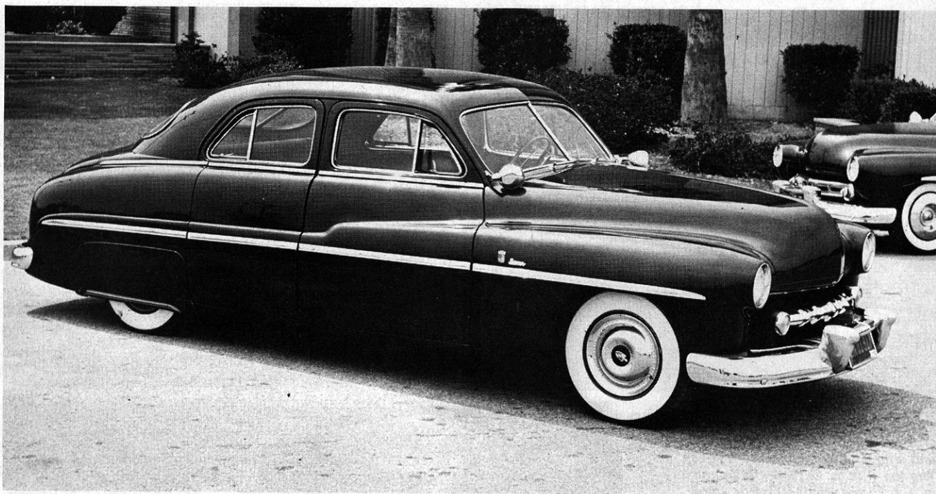
Two 4-door Mercs by Barris—a 1949 mildly customized, and a 1950 with chopped top, drip rails removed and a 1949 DeSoto rear window to replace the larger original unit. Both cars have door handles removed, are de-chromed and lowered. Interior is of chopped '50.
