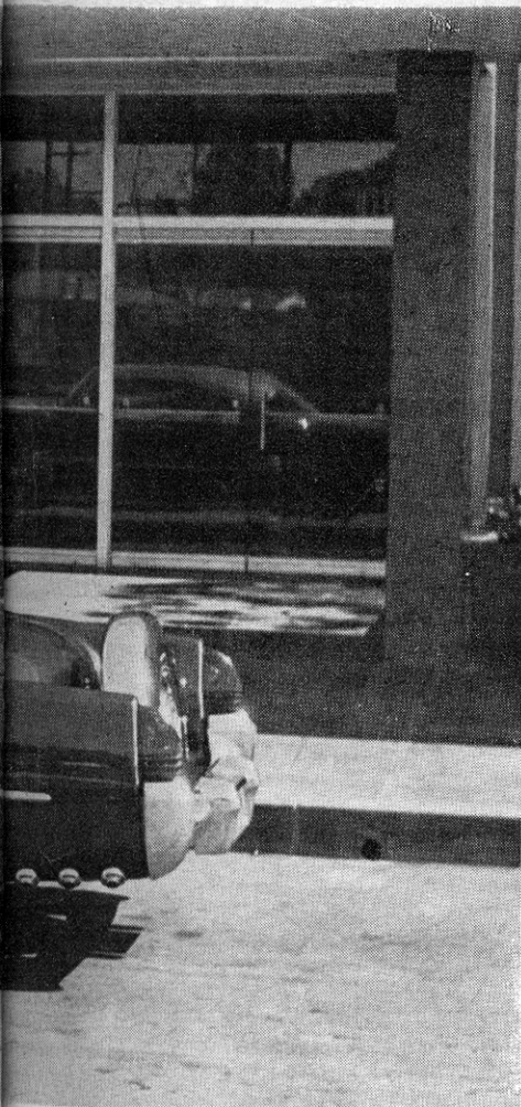
Extended fenders go past continental mount and fair neatly into the body. Valley Custom built license light mount which is set on rear bumper instead of the tire
